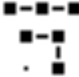
Fig.7 The only two possible topologically different avalanche configurations with s=3 . Black squares indicate the flipped spins, the lines indicate the bonds between them
